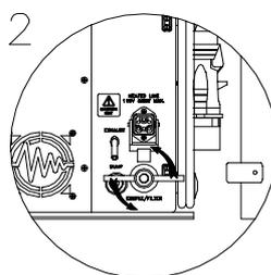
Push in and turn the tool 90 degrees anti-clockwise
