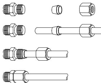
Figure 2 Tube Fitting Assembly
