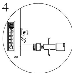
Pull out the filter retainer and sample filter. Replace or clean the filter.
