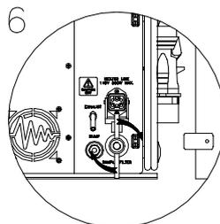
Push filter and filter retainer into the MINIFID with the T-bar vertical, then rotate the tool 90 degrees clockwise to lock the filter retainer in position
